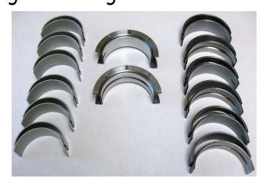
TRE529318 Con Rod Brg Std (Pair)TRE529319 Main Brg Std (Pair)TRE529320 Thrust Brg Std (Pair)
